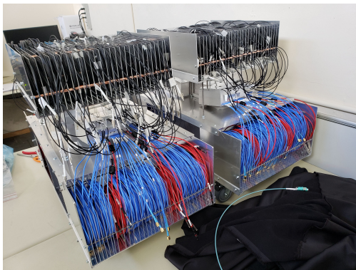
(a) FT0-C test assembly for MCP-PMTs in the FIT Lab.
